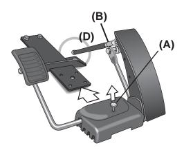
1. Pull the release button (A). Slide the LFA unit onto the mounting plate, placed on the floor, so that the mounting plate runs **through** the LFA unit.
