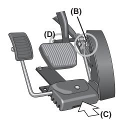
in along the mounting plate **(C)** so that the catch can lock the unit as you let go of the release button. This will be heard as a click-sound.
