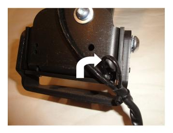
2. Use a sharp tool to test movement of upright and slider. Make sure they slide freely and return to normal position.
