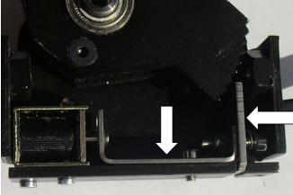
3. Check 2 screws under base that holds solenoid from moving.
